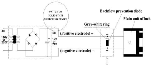
Connection method of backflow prevention diode:
