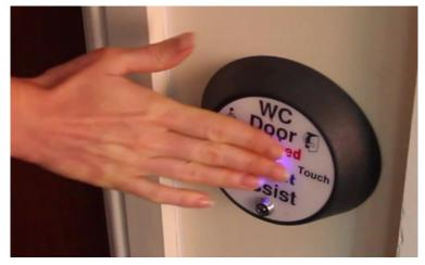
**Step 2** - Once inside the toilet and the door has fully shut behind you, touch the inside sensor (which will look like the pictures below). The door will lock and the light will turn red to indicate that it is locked.
